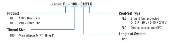
**NOTE:** Nominal power output of Rizer-Line system is 3 W/ft @ 50°F (10 W/m @ 10°C) or 5 W/ft @ 50°F (16 W/m @ 10°C). Only available in Drinking Water Safe Fluoropolymer outer heating cable jacket.
