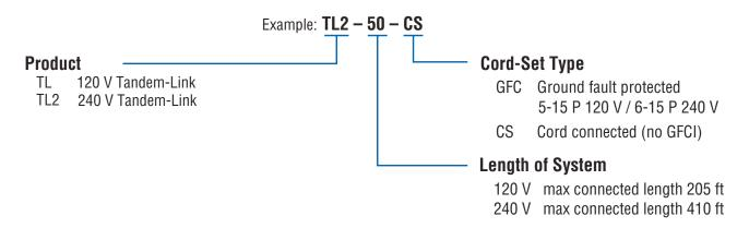
NOTE: Nominal power output of Tandem-Link system is 5 W/ft @ 50°F (16 W/m @ 10°C). Only available in Modified Polyolefin outer heating cable jacket.
