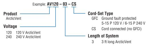
NOTE: Nominal power output of ArcticVent system is 75 W/ft @ 50°F (10°C).
