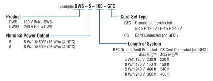
NOTE: Installers must provide 20 Amp circuits for CS circuit lengths greater than 460 ft for 5 W/ft and 300 ft for 8 W/ft systems.
