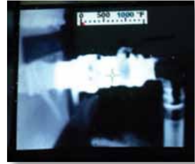
▲ Thermal image showing the heating effect of freeze protection on the 2 1/2" discharge valve
