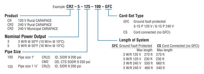
**NOTE:** For "CS" system installers must provide 20 Amp circuits for circuit lengths greater than 550 ft for 3 W/ft CARAPACE and 460 ft for 5 W/ft CARAPACE.
