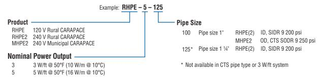
NOTE: Installers must provide 20 Amp circuits for circuit lengths greater than 550 ft for 3 W/ft CARAPACE and 460 ft for 5 W/ft CARAPACE.
